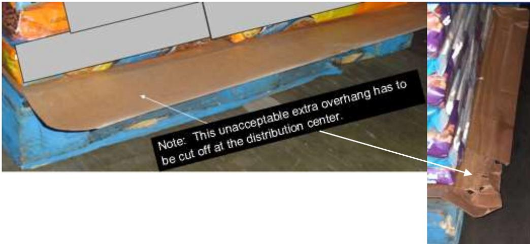
Dollar General prefers a stacking height of 68 inches (including the pallet) unless it prevents cubing out the trailer. Product should not extend over the edge of the pallet and should have only one SKU per pallet unless accompanied by a “Mixed Skid Sheet” documenting the items contained on the pallet. Pallet loads should not exceed 2500 pounds. Purchase orders and lots must not be mixed on a pallet or slip-sheet.
