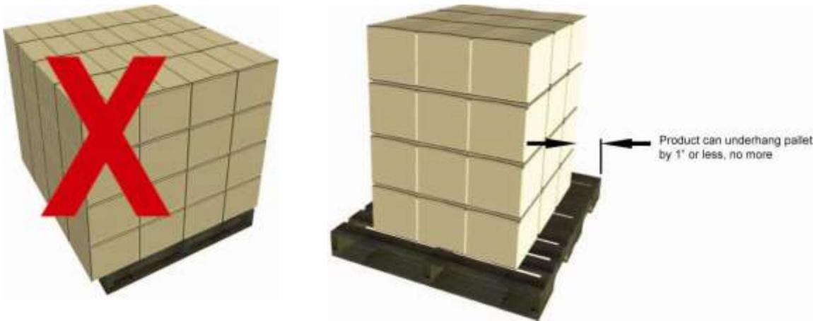
All unit loads must arrive intact and be able to be easily taken from the trailer without unit failure. Unstable loads must be secured with airbags, dunnage, etc. to prevent unit shifting during transit. Refer to the Transportation Section for more details about securing the load.
