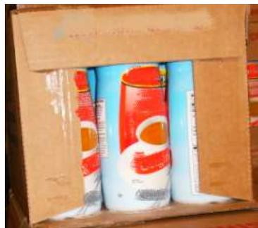
Crushed packaging may contain damaged product and/or make stacking of the packaging dangerous.
